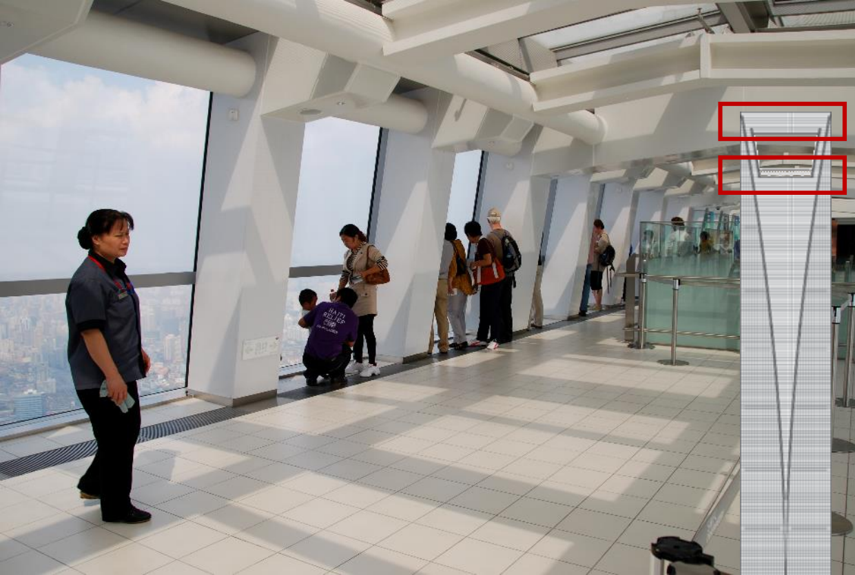
Shanghai World Financial Center has two observatory levels separated by a large void. The upper level is narrower and slopes the glass to make view down easier.
